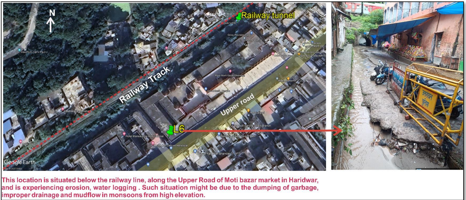
Fig 7: Google Earth image shows the location L6, situated just below the Haridwar railway track. It is observed that the area around L6 experiences a water logging situation that has led to an erosive effect on the surroundings and adjacent to the market area. The location point on the Google Earth image is explained with respect to field photographs.
